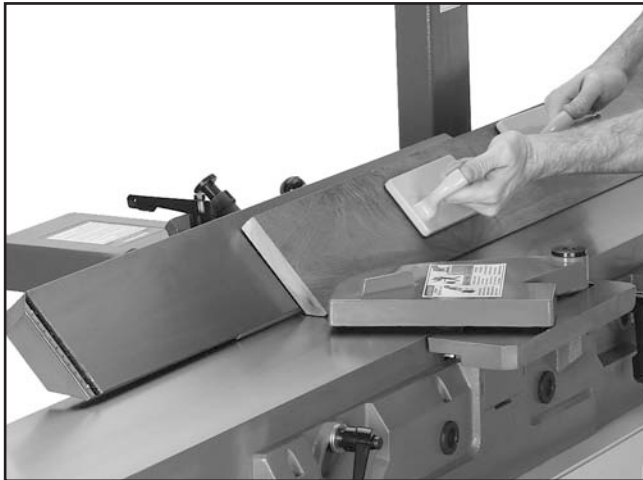
Figure 29. Fence setup for a bevel cut of 45°.
